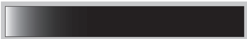
Figure 4: Part of Fresnel reflection intensity: (1-x)^5 where x is expected to be \cos(\theta)
