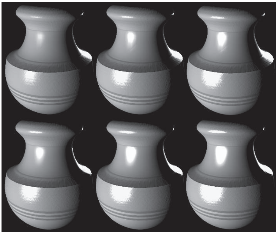
Figure 15: Rendering with various refraction index values with pixel shader 1.4 (top row) and pixel shader 2.0 (bottom row). Roughness is constant at 0.15. The index of refraction is 0.15, 0.45, and 0.85 (left to right). Note the visibility of the face edges and error (crack) in the middle of the large highlights in the 1.4 version. (See Color Plate 1.)
